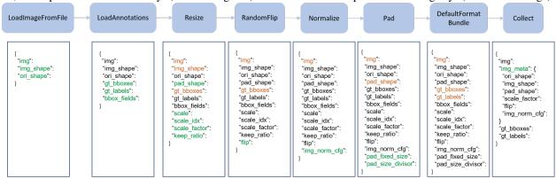
Here is a pipeline example for Faster R-CNN.
