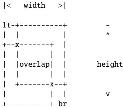
To ensure IoU of generated box and gt box is larger than `min_overlap`:
