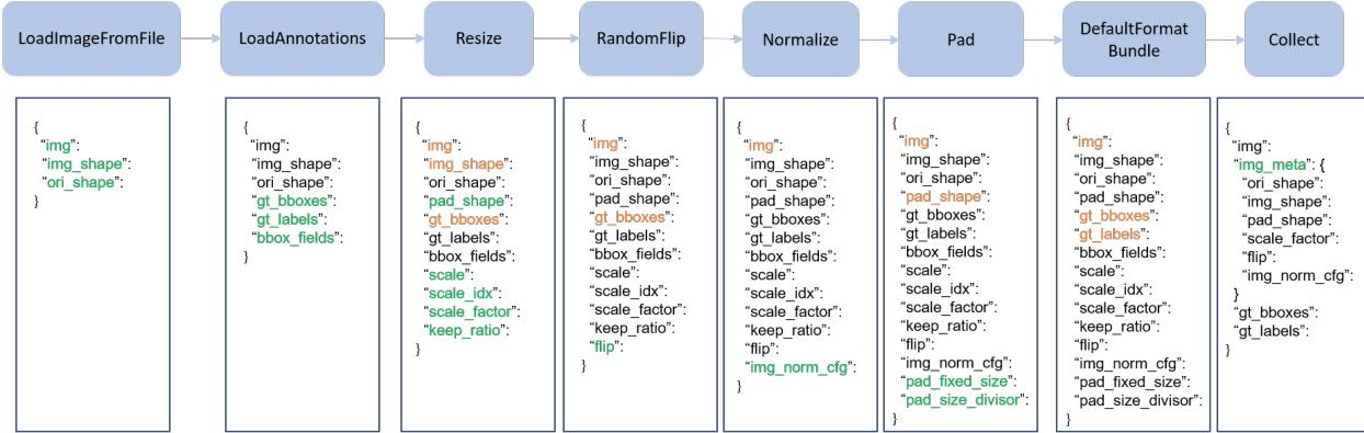
The operations are categorized into data loading, pre-processing, formatting and test-time augmentation.
